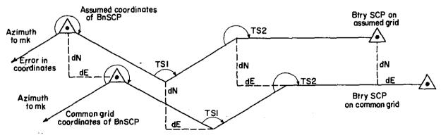
Figure 142. Sliding the grid.
