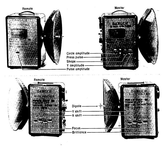
Figure 17. Side views of master and remote units.
