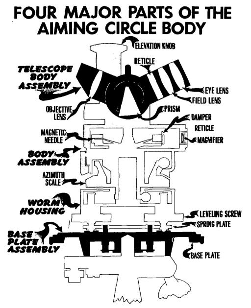
Figure 30. Cutaway drawing of aiming circle showing composite parts.
