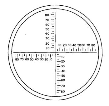
Figure 31. Telescope reticle.
