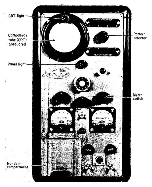
Figure 15. Control panel, master unit.
