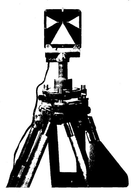
Figure 46. Tripod-mounted target.
