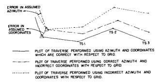
Figure 141. Discrepancies in survey control caused by use of assumed starting data.
