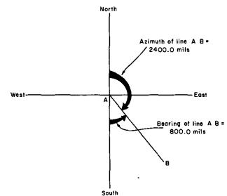
Figure 50. Relationship of azimuth and bearing.
