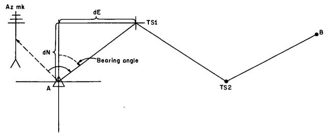
Figure 52. Requirements for dE and dN.
