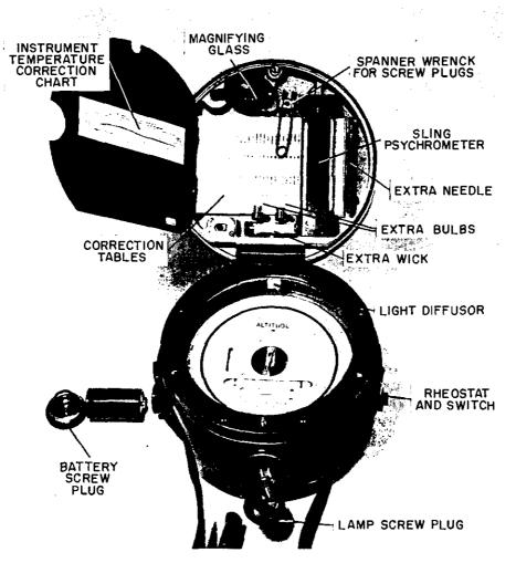
Figure 90. Surveying altimeter, 4,500-meter, 2-meter divisions.
