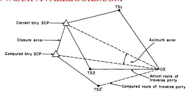
Figure 65. Azimuth error.
