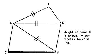
Figure 73. Route of trigonometric height computations.
