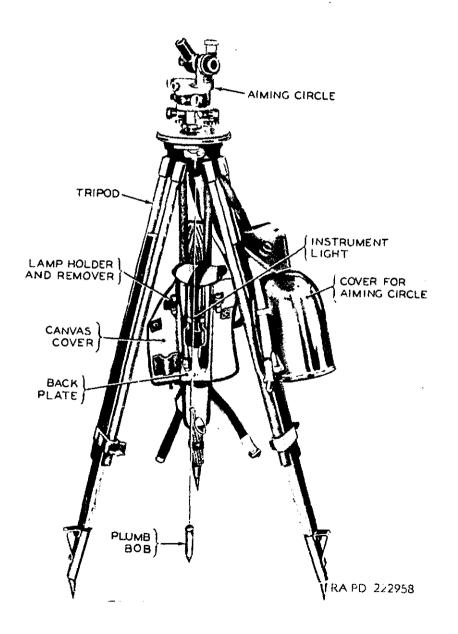
Figure 29. Aiming circle with accessory equipment.
