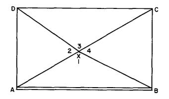
Figure 81. Central point quadrilateral.
