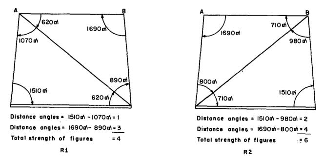
Figure 78. Determination of R1 and R2 chains.
