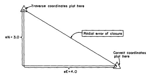
Figure 61. Radial error of closure.
