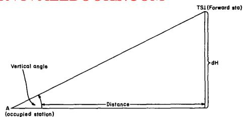
Figure 54. Right triangle for determination of dH.
