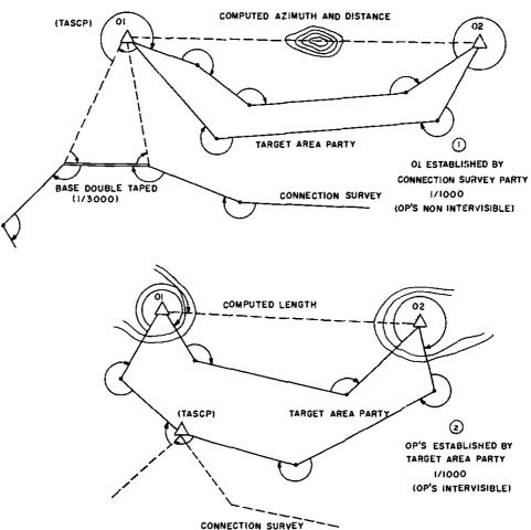
Figure 1. Target area base survey.
