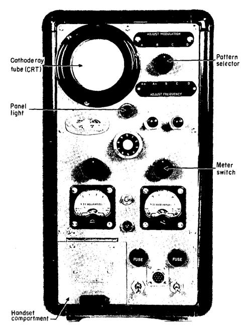
Figure 16. Control panel, remote unit.
