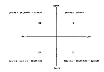
Figure 51. Determination of bearing angle.
