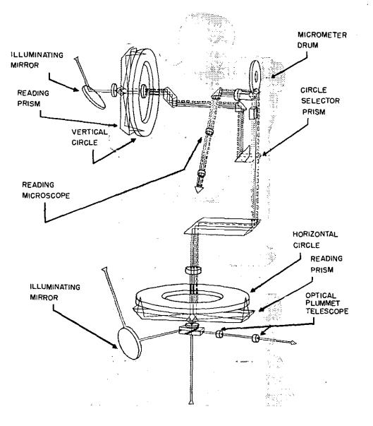
Figure 39. Circle-reading optical system of the T2 theodolite.
