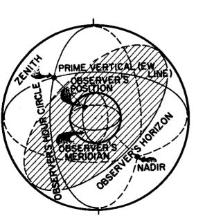
Figure 110. Elements relative to observer's position.
