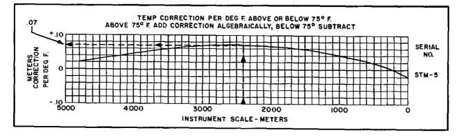
Figure 93. Instrument temperature correction chart.
