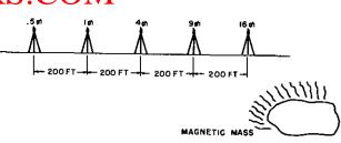
Figure 104. Detecting hidden magnetic disturbance.
