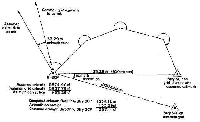
Figure 143. Swinging the grid for a specific station.
