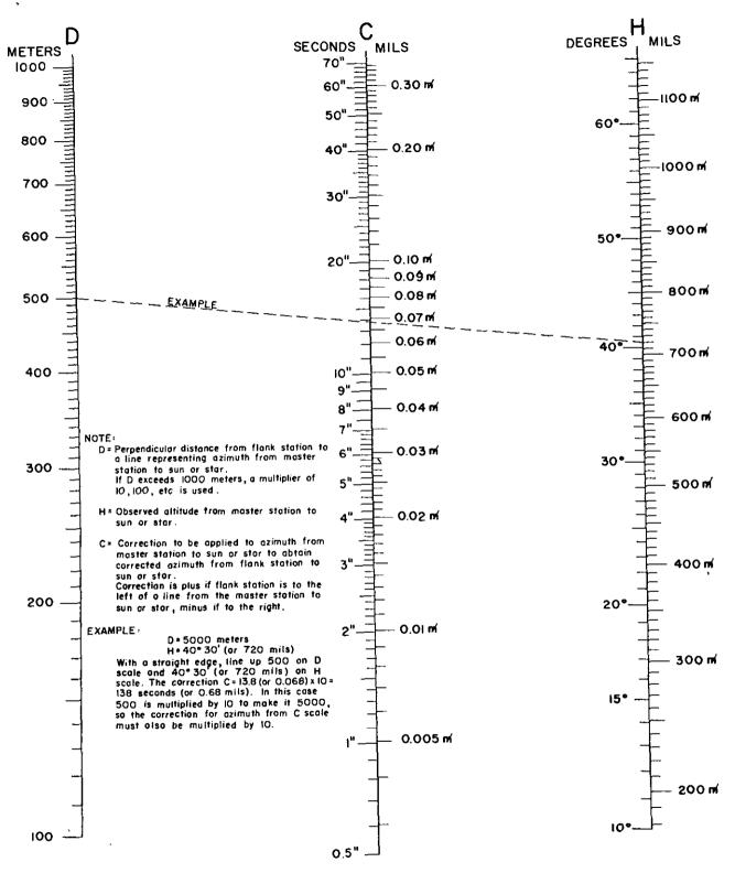
Figure 108. Simultaneous observation, grid azimuth correction nomograph.
