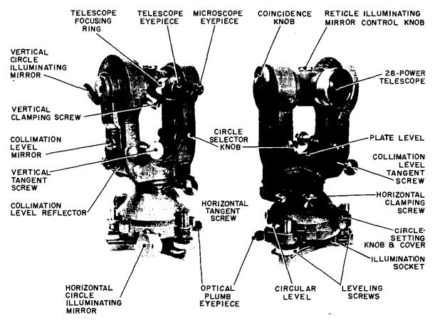
Figure 38. The T2 theodolite.
